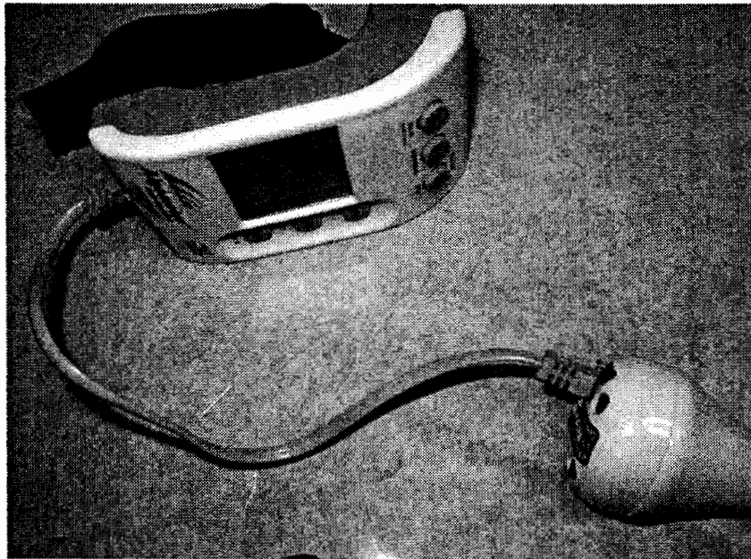
Figure 9. Pressure threshold algometer. The 0.5cm contact-tip is illustrated in Figure 10.
